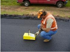
**Calculating unit weights for input into density gauges**
