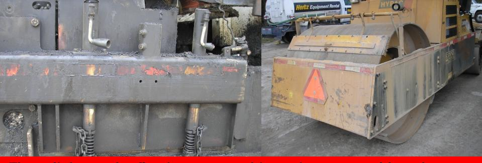
These lights and reflective tape on this equipment would not be seen well, if at all, at night. Wipe the lights and tape with a clean rag.
