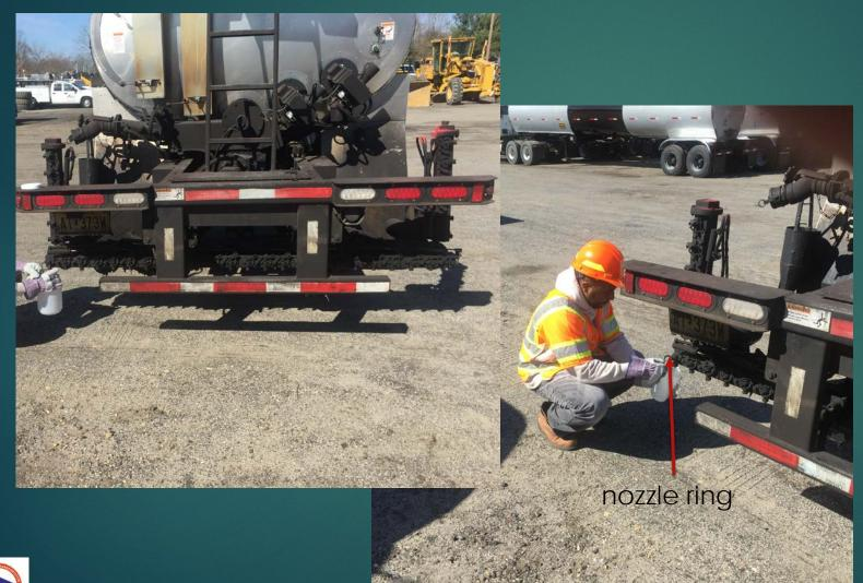
Allow at least 20 yards to run out before taking sample. Pull the nozzle ring to collect sample.
