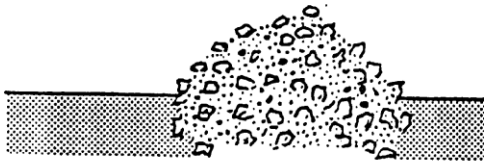
3 Dispersions of hard particles in a softer matrix
