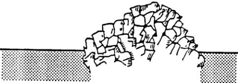
4 Materials which fracture in an irregular angular manner
