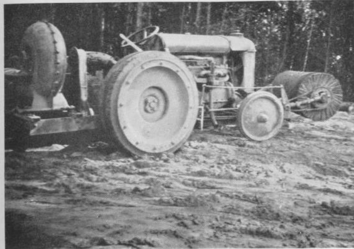
ROAD CLEANING EQUIPMENT, SHOWING BROOM AND BLOWER MOUNTED ON A FORDSON TRACTOR. THE BLOWER REMOVES THE DUST THAT HAS NOT BEEN ENTIRELY SWEEPED OFF BY THE BROOM.
