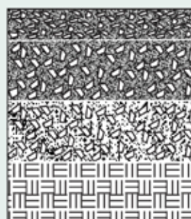
HMA on Aggregate Base
