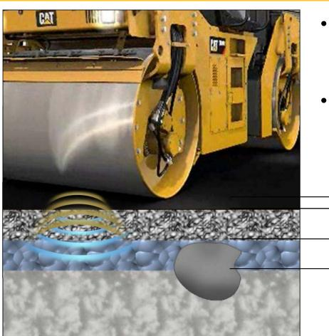
Accelerometer measures deeper than the lift of asphalt being paved
