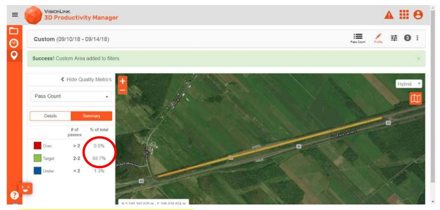
Breakdown rollers only: 99% > target pass for breakdown
