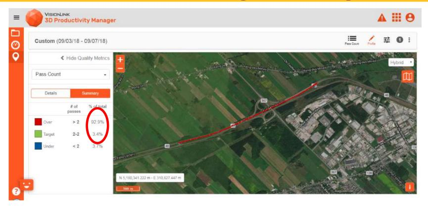
Breakdown rollers only: 96% > target pass for breakdown
