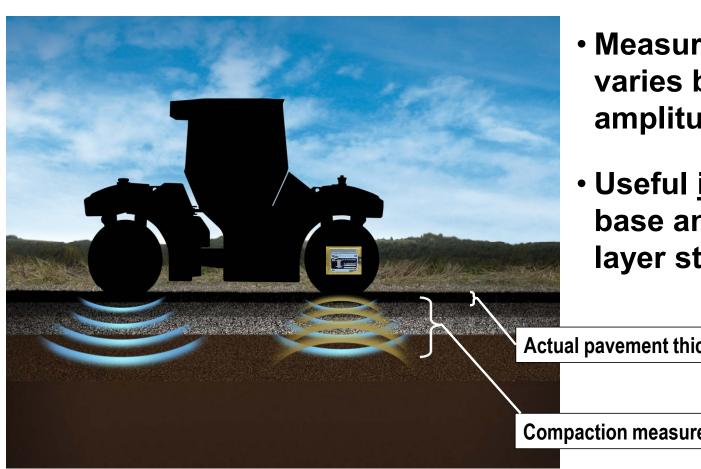
Measurement depth varies based on amplitude setting
