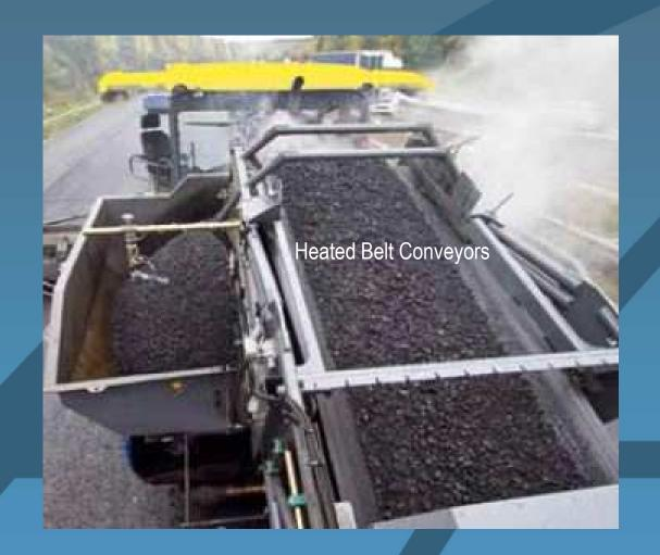
Material is delivered in a homogeneous mass.
