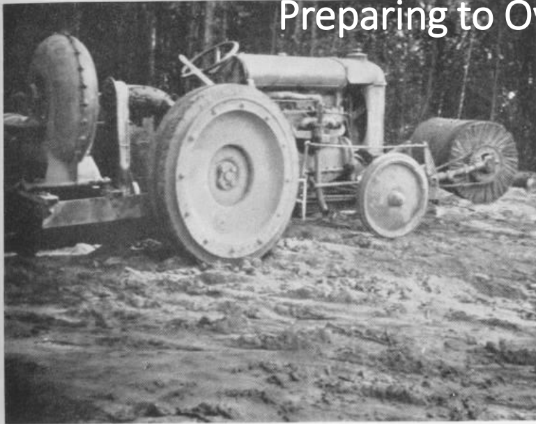
ROAD CLEANING EQUIPMENT, SHOWING BROOM AND BLOWER MOUNTED ON A FORDSON TRACTOR. THE BLOWER REMOVES THE DUST THAT HAS NOT BEEN ENTIRELY SWEEPED OFF BY THE BROOM.
