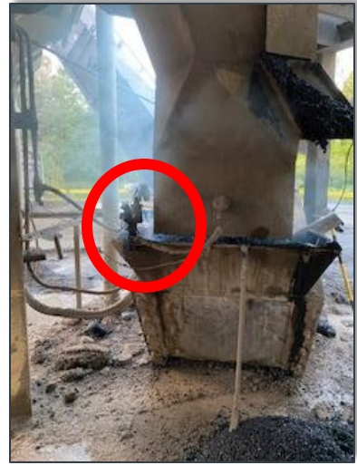
One particulate analyzer placed over the chute
